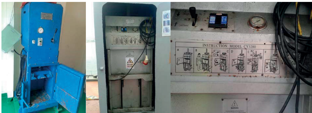
Example of compacters. Source: Maritime Administration of Bulgaria
