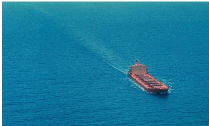
Discharge of coal cargo residues trailing vessel. Source: Australian Maritime Safety Authority
