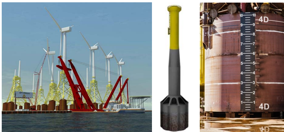
Figure 10: Left: Suction Installed Wind Turbine (SIWT) of SPT Offshore (source: SPT Offshore, Woerden NL). Middle: Multi-shell concept of Universal Foundation (2013). Right: Suction buckets for the substation at Global Tech 1 (Source: Global Tech 1 2013).
