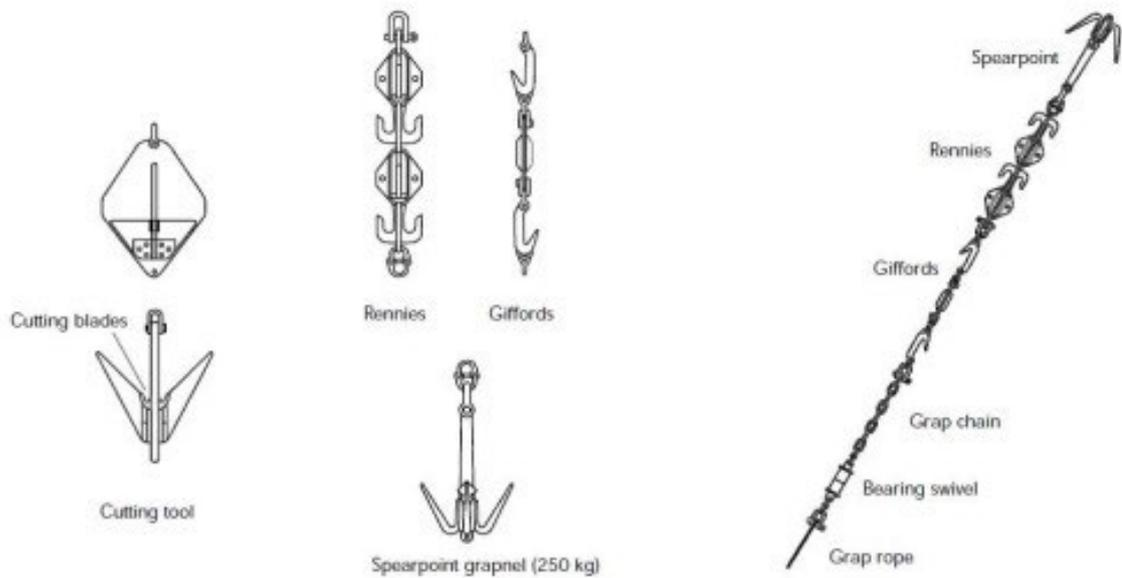
Figure 10 Diagram of Grapnels. Image courtesy of Alcatel Submarine Networks
