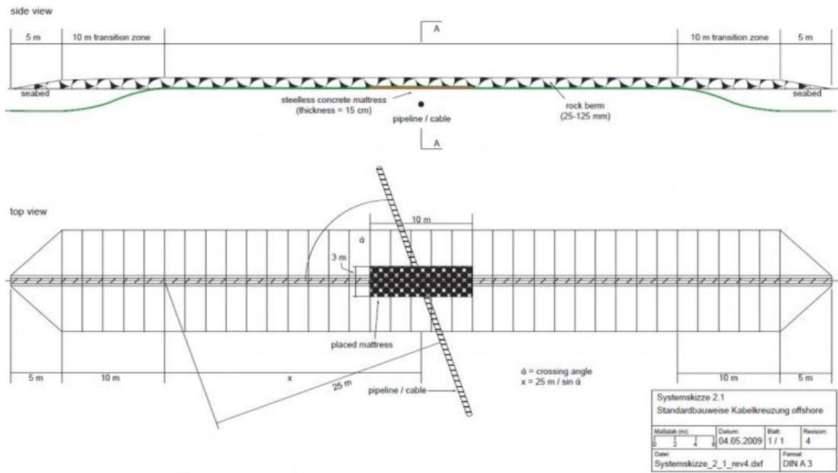
Figure 132 : Example Design of Power Cable Crossing Over Existing Cable: Image TenneT Offshore GmbH.
