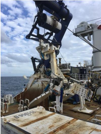
*Figure 15 Skid Supported SLB Power Cable Plough - Prysmian's Heavy Duty Plough : Image D. Sinclair TenneT Offshore GmbH*
