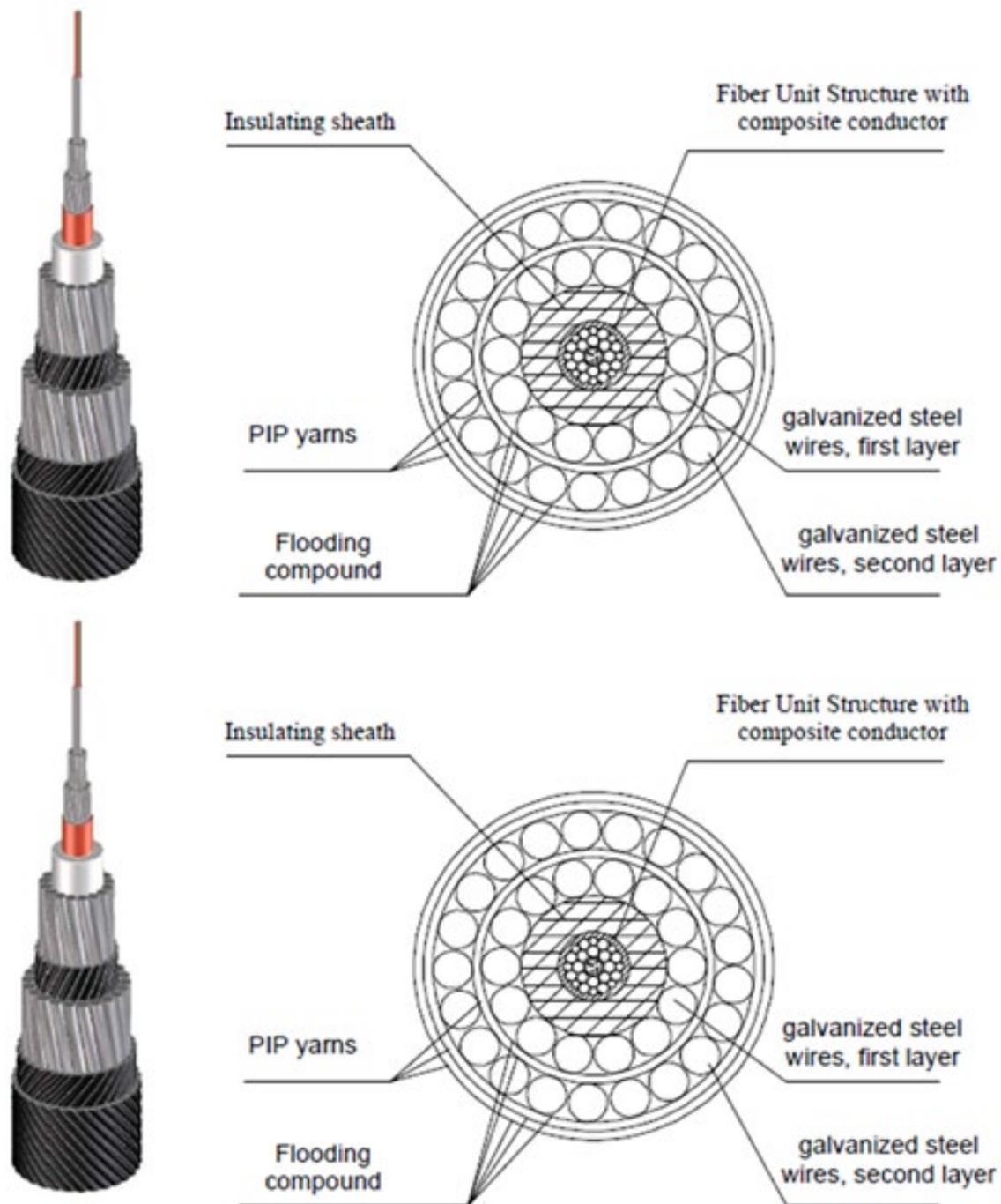
Figure 3 Diagram of Double Armour Telecommunications Cable. Indicative diameter range 37.5mm-50mm dependent on cable type. Image courtesy of Alcatel Submarine Networks.
