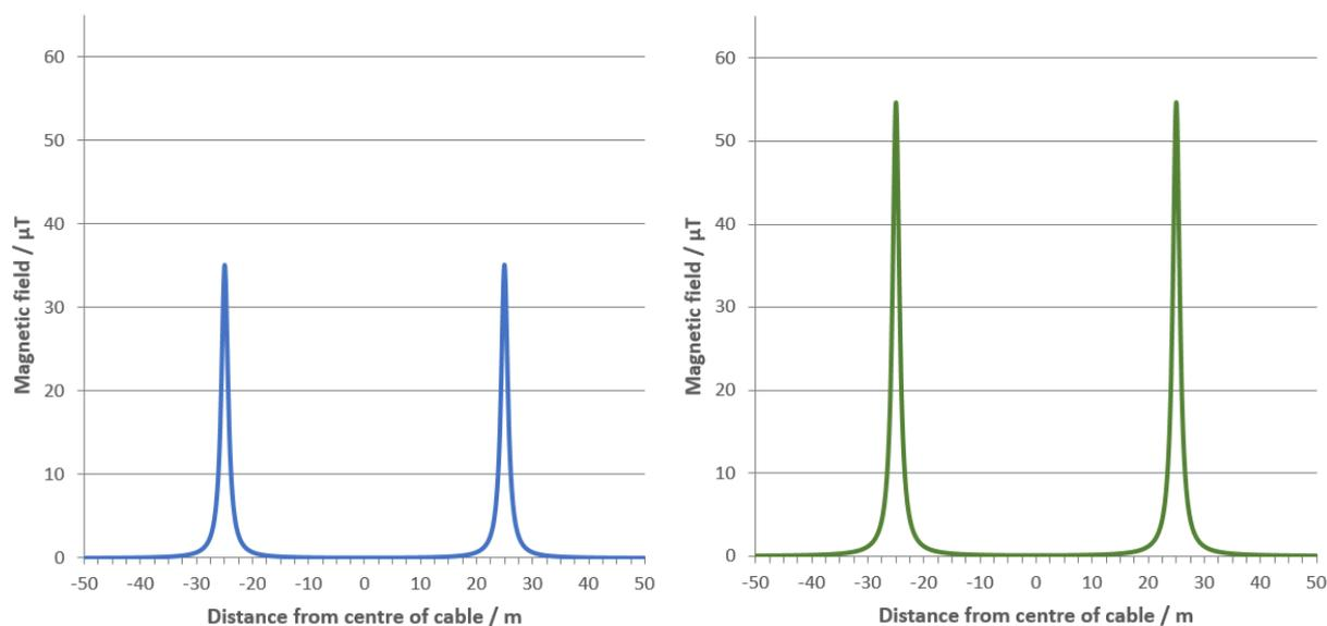
Figure 8: Maximum Calculated AC Magnetic Fields.
