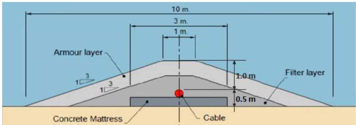
Figure 14 : Typical Rock Berm Profile at Crossing: Image TenneT Offshore GmbH
