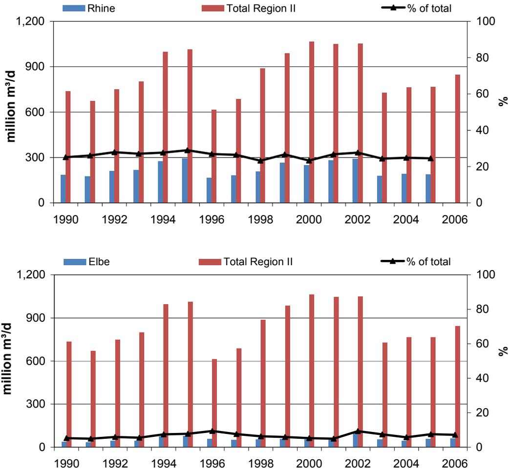
**Figure 4.13:** Annual total river water discharge 1990 – 2006 to Region II (red bars in both charts), river Rhine (blue bars in the upper chart) and Elbe (blue bars in the lower chart). The relative shares (% of total) of Rhine and Elbe to the total water discharge in Region II are indicated by a solid line.
