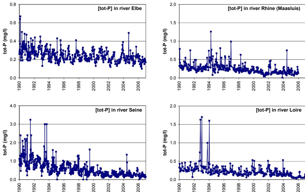
**Figure 5.17:** Observed concentrations of total phosphorus at the four rivers/sites with a significant decline in riverine inputs of total phosphorus. The missing values for Loire in 2005 and 2006 were interpolated
