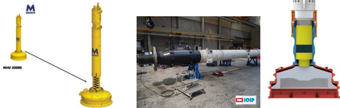
Fig. 7. View of a standard hydraulic impact hammer and a modified hammer (right) with a MENCK Noise Reduction Unit (MNRU) added between ram weight and anvil (left, © MENCK) and IHC S-90 hammer with added PULSE system in black housing (middle) and cross-sectional view (right, © IHC IQIP).
