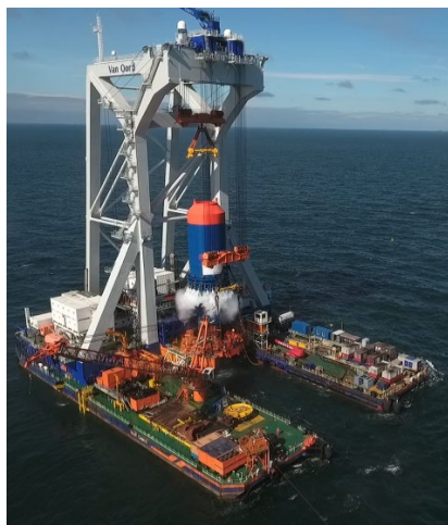
Fig. 8. Draining of seawater from BLUE 25M hammer upon completion of piling operation (left). Frequency spectrum of BLUE piling compared to impact piling at two reference piles (right, note different dimensions: BLUE Piling test: \varnothing 6.5 m, water depth 22 m; reference Gemini OWF: \varnothing 6.6 m, water depth 30 m; reference Q7 OWF: \varnothing 4 m, water depth 19-24 m), © Fistuca BV.
