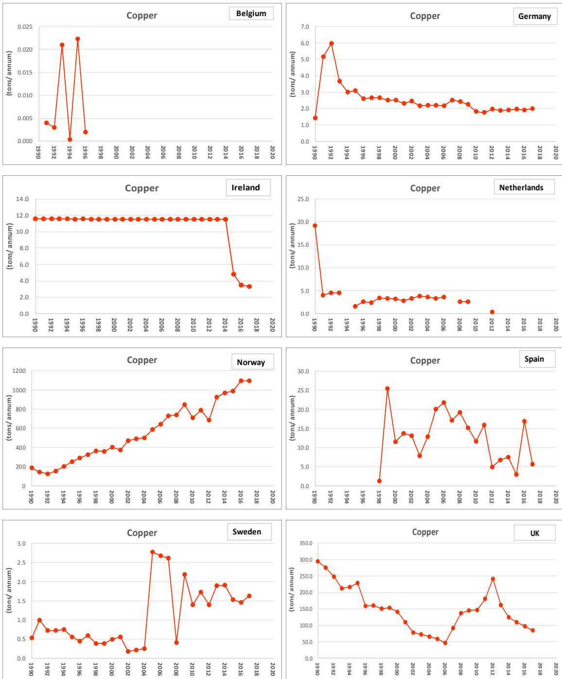
Figure 3d. Direct discharges of copper (Cu) from eight Contracting Parties (Belgium, Germany, Ireland, the Netherlands, Norway, Spain, Sweden, and UK) in the period 1990-2017. Note that the scales on the y-axis are different.
