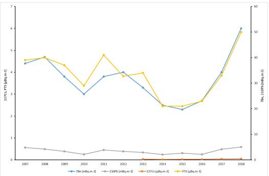
Figure 6 - Temporal variation of the activity concentration of <sup>7</sup>Be<sup>210</sup>Pb and Cs<sup>137+'«'c-c-</sup>and concentration of suspended particles (µg.m<sup>-3</sup>) in aerosols collected at CTN.
