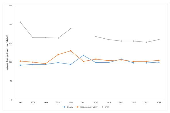
Figure 10 - Average values of the flow rate equivalent of the ambient dose measured at each measurement point in the CTN in each quarter and the respective annual average value (values expressed in nSv.h-1).
