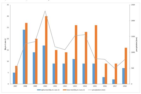
Figure 7 - Temporal variation of total alpha and beta activity resulting from atmospheric deposition and precipitation values at CTN.
