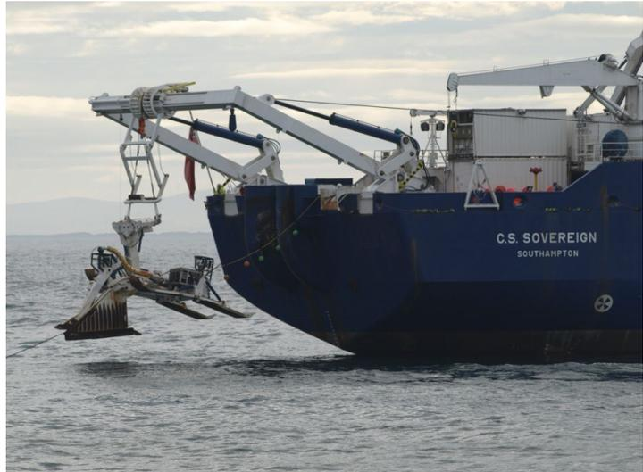
*Figure 16 Telecommunications cable plough being deployed on an 'A Frame'. Image Global Marine Group.*
