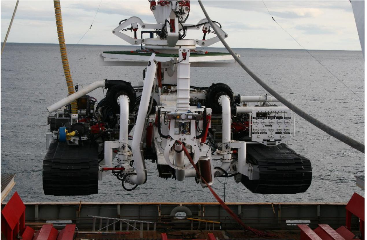
Figure 187 Example of A Post Lay Burial Chain Cutter Tool – Canyon’s I-Trencher : Image D. Sinclair TenneT Offshore GmbH.
