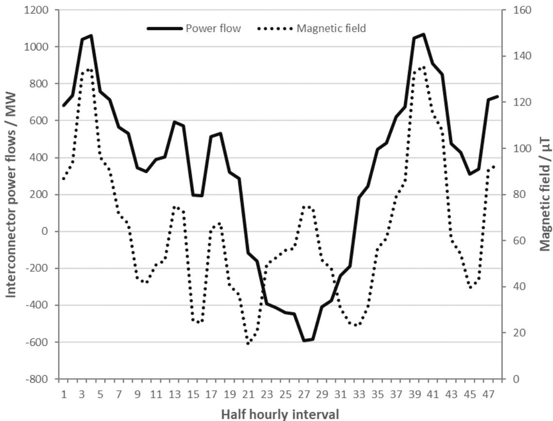
Figure 6 : Power Flow<sup>7</sup> And Magnetic Field Changes Over A 24-Hour Period From A HVDC Interconnector Between the UK And Norway. Cables Buried 1.5m Below Seabed. Calculations Of Magnetic Field at Seabed.
