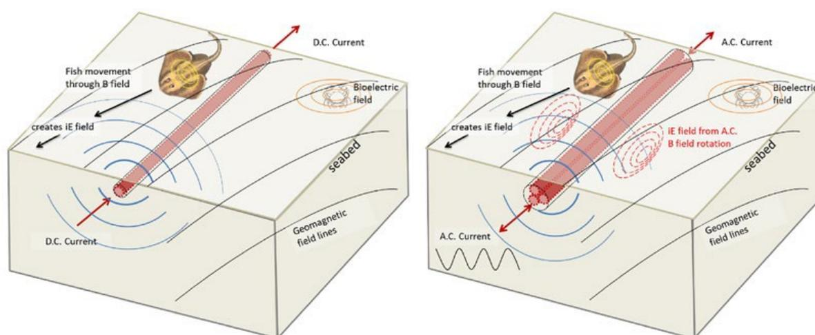
Figure 21: Schematic diagrams of natural and anthropogenic electromagnetic fields including magnetic (B-fields), electric (E-fields) and induced electric fields (iE-fields). This figure is intended to show differences in the electric fields and their spatial footprint related to DC and AC cables (as also illustrated in Figure 7 and 8). Left: DC-cable, right: AC-cable. From GILL & DESENDER (2020) (adapted from NEWTON et al. 2019).
