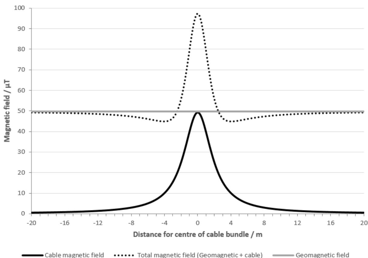
Figure 7: The Calculated Magnetic Field from A Bundled Bipole System With Cables Orientated North South and Its Combination with The Earth’s Geomagnetic Field
