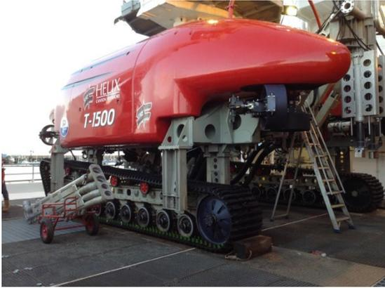
*Figure 176 Example Of A Power Cable Post Lay Burial Jetting Tool - Canyon's T-1500 : Image D. Sinclair TenneT Offshore GmbH.*
