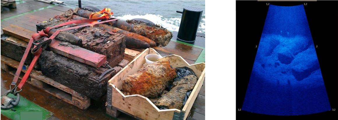
Figure 11 *Acoustic Survey of UXO Items (Right). Safely recovered items (Left)*
