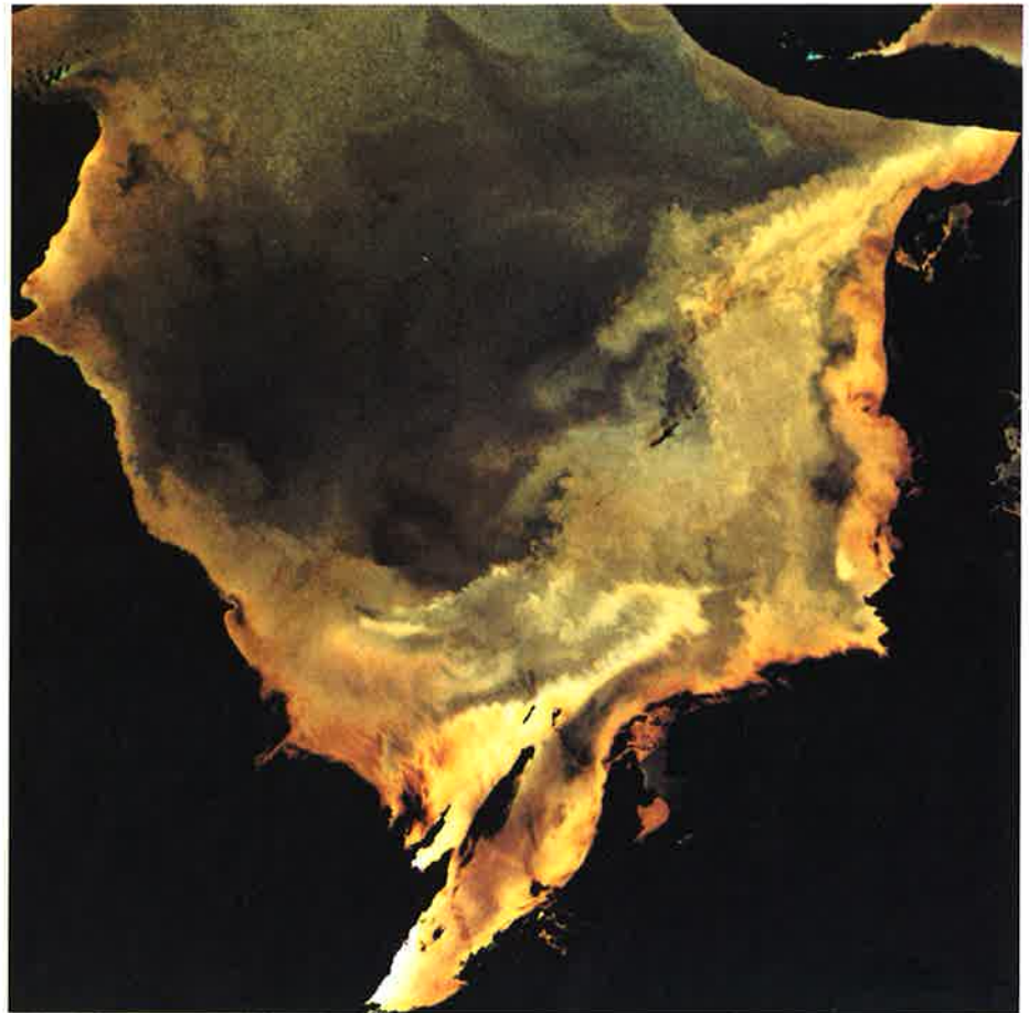
Figure 2-17. Transport of solids and circulation patterns in the North Sea. Nimbus-7 satellite CZCS colour composite image obtained in March 1982, showing suspended matter distributions, and absorption by chlorophyll and dissolved organic matter. Source: Aiken (1989).
