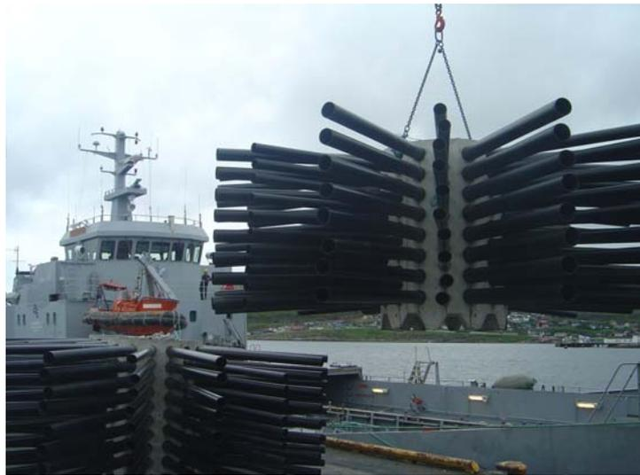
The cylinder is filled with stones to increase weight and stability. From the cylinder 14 vertical rows of 2.5m long polyethylene pipes – with a diameter of between 9 and 18 cm – radiate outwards. Together, the cylinder and plastic pipes on each unit provide an external and internal surface area of 250m<sup>2</sup>, the pipes provide 300m pipe length, and the total weight is 9 metric tonnes.
