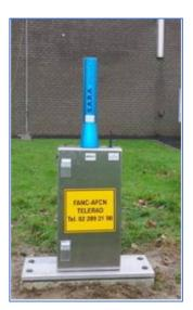
**Gamma spectrometry stations** (about 65) for measuring the <u>ambient gamma radioactivity and</u> <u>the gamma radioactivity of certain radionuclides</u> (<u>10 predefined nuclides</u>), are distributed on the fences around all nuclear sites and in the agglomerations (~ 5 km around the site) of the Nuclear powerplants Doel and Tihange. Photographs show a station in its environment.
