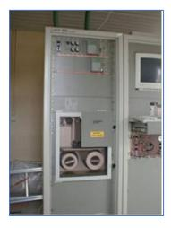
The photograph on the left shows the alpha/beta measuring unit with a view of the unreeling filter tape which collects the dusts and particles impacted when the air is pumped.
