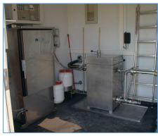
Inside is the gamma spectrometry unit housed in its own tank, surrounded by a strong lead screen protected by a stainless steel casing in which the water pumped from the river enters and leaves – photograph on the left. Ten radionuclides are defined in the recognition software.
