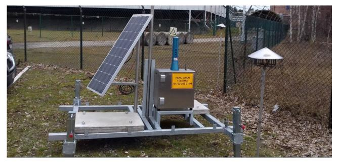
The **aerosol stations** (ZnS detector), of which there are 7 for measuring the <u>radioactivity of dusts</u> suspended in the air (aerosols and fine particles), which determine the <u>total alpha and total beta</u> radioactivity.
